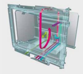
the firebox towards the fire bed. This stream of air is under the same valve control as the conventional secondary air. When the stove is running at its nominal or rated output the dual secondary air system ensures effective mixing of the fuel and combustion air. This reduces the amount of air required which in turn improves efficiency and reduces
