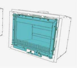
For easier installation of the R5 and R6 we have developed a convection chamber that can be fitted as a separate unit from the firebox. Additionally, the flue collar can be fitted at either a 30° angle or vertical, depending on the specific needs of the installation.
